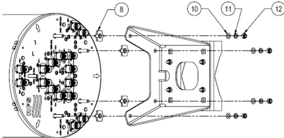
3. Connect item 3 to above sub-assembly by M12 screw, washer and nut (No need to tight).
