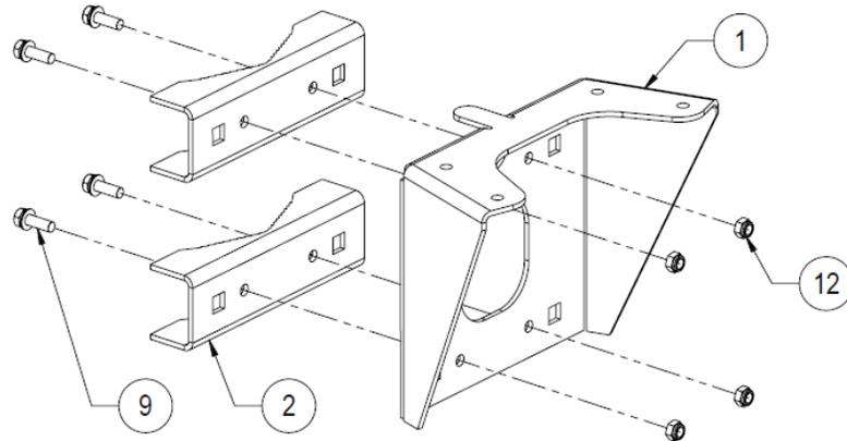
2. Assemble above sub-unit and item 8 to antenna by M8 washer and nut (with 11Nm / 8 ft-lbs torque). **NOTE: The convex steeliness ring on item 8 MUST be inserted to end plate of antenna.**
