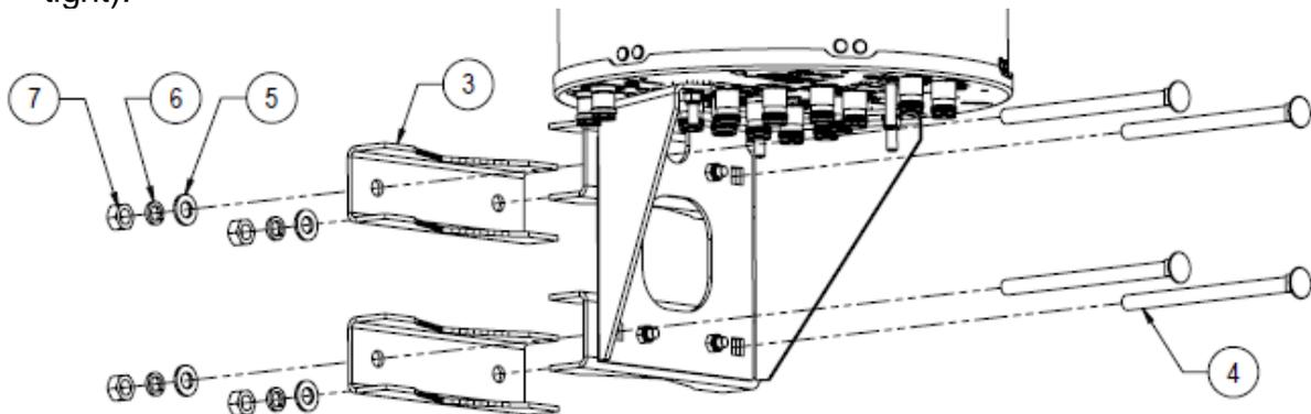
4. Insert the full assembly to pole (*diameter between 60 mm & 120 mm*) and tight M12 nut with 40 Nm / 30 ft-lbs torque.
